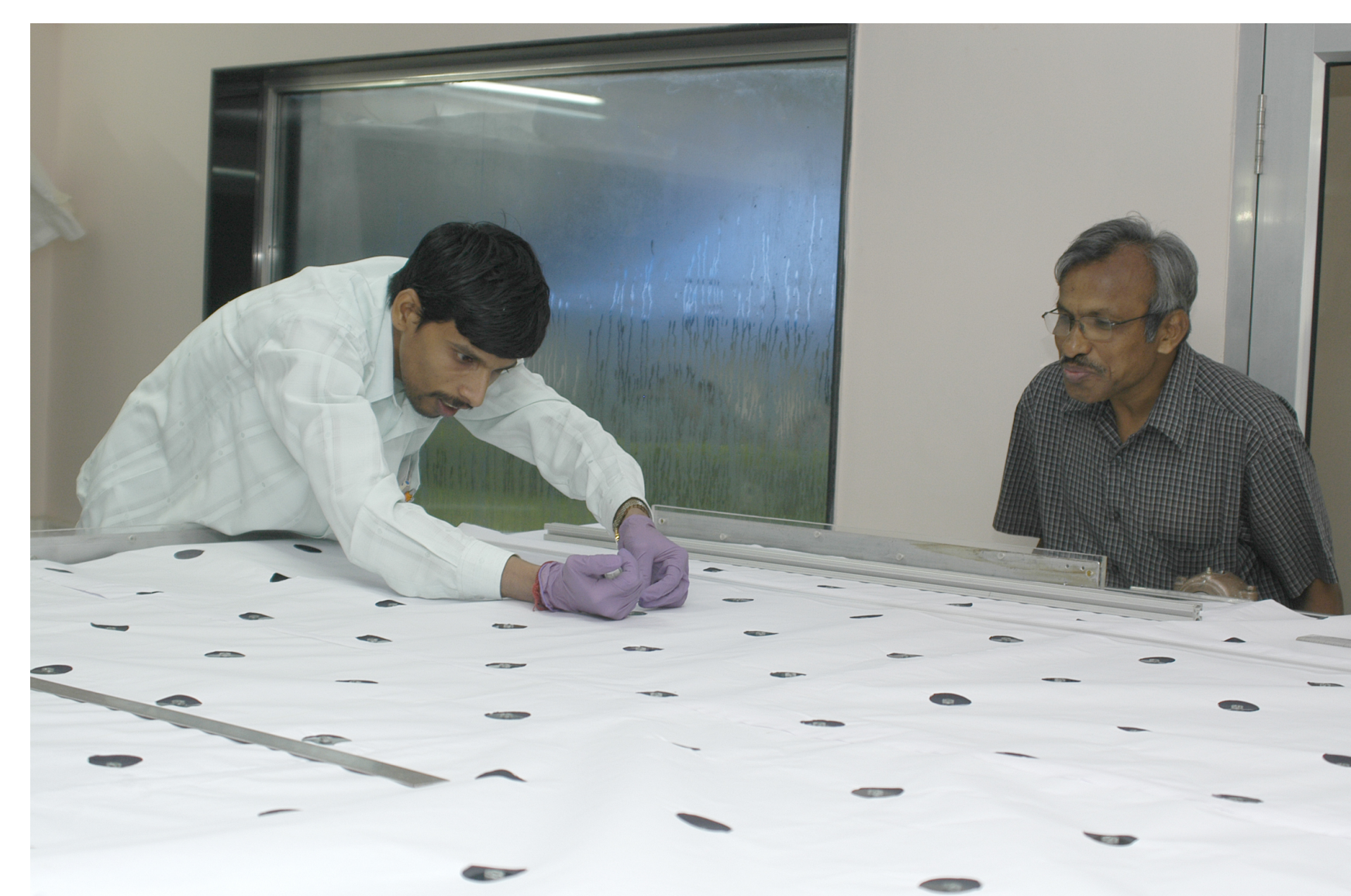
Figure: RPC fabrication in process at TIFR.
