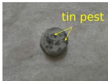
Figure A.2: 0.1% Sn-In (In by mass %) shows signs of tin pest after 3 warming and cooling thermal cycles in the CFDR-1200.
