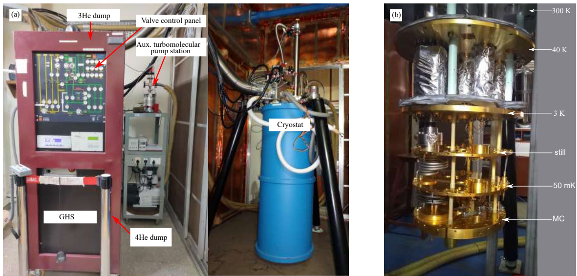
Figure 2.4: The Cryogen Free Dilution Refrigerator (CFDR-1200) at TIFR Mumbai: (a) The gas handling system (GHS) and the cryostat (b) The thermal stages of the cryostat, which are visible after removing the thermal and vacuum shields.
