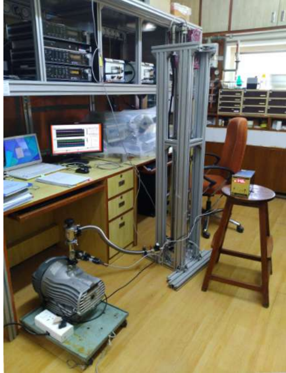
Figure 2.13: Initial vacuum test of the probe lift.
