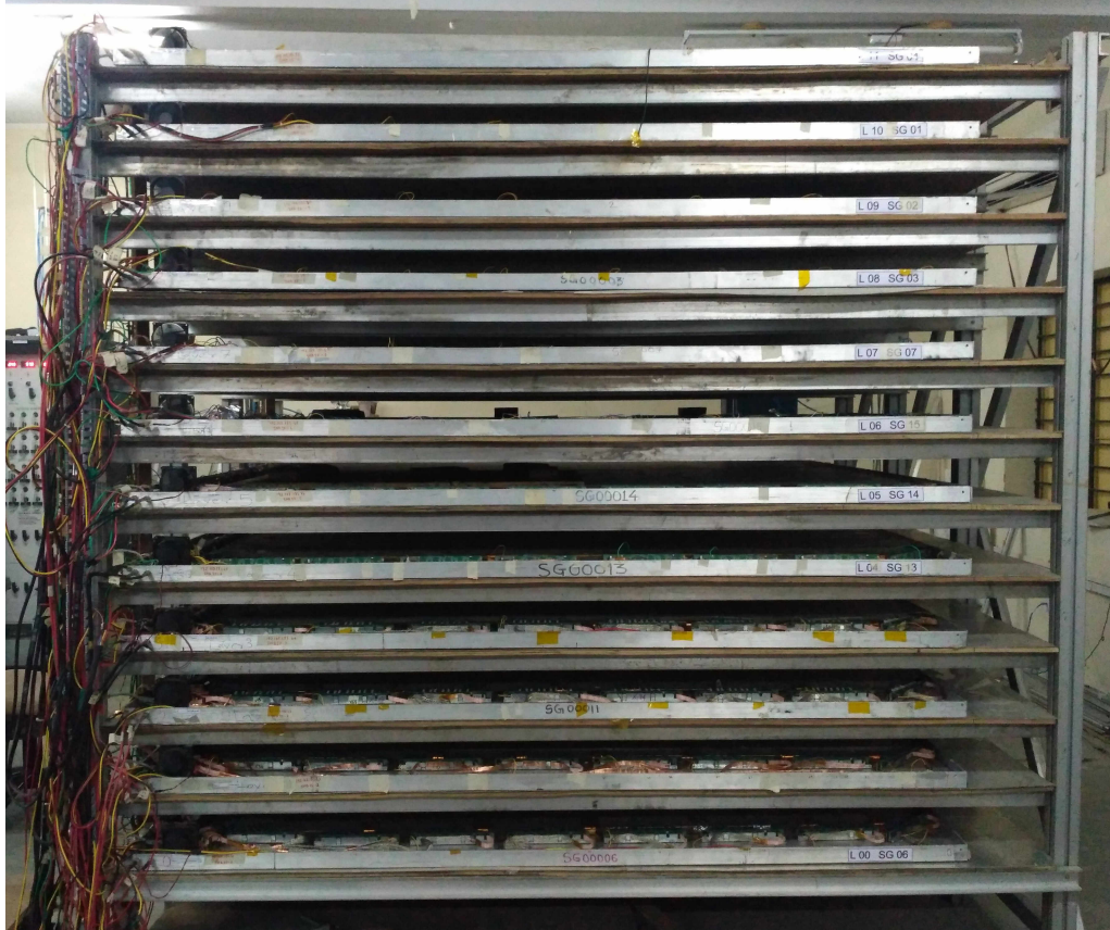
Figure 1.5: Detector Stack with 12 Layers of 2\text{ m} \times 2\text{ m} RPCs.
