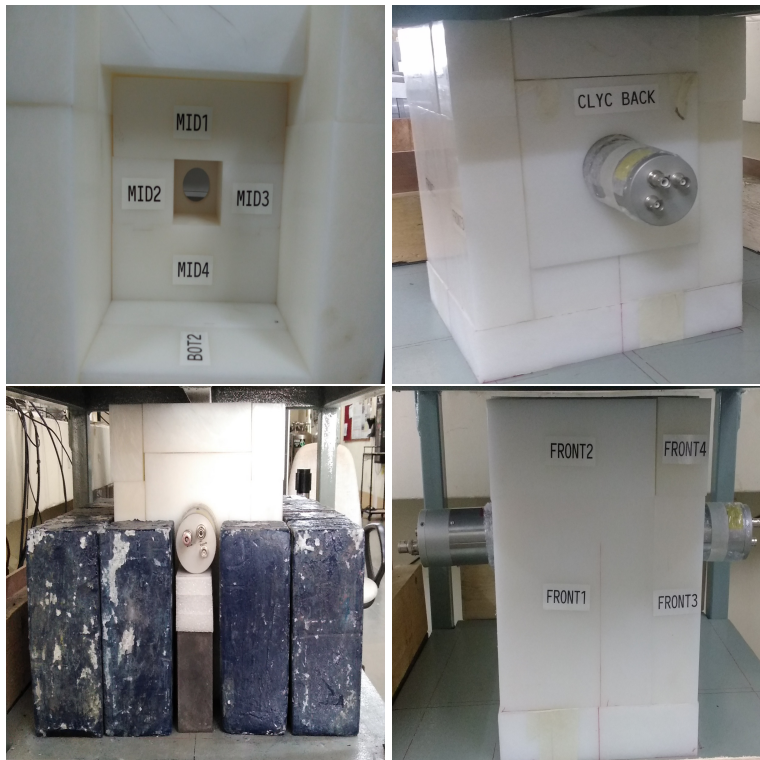
FIGURE 3.2: Clockwise from the top: 1. The inner view of the HDPE, 2. view of CLYC detector mounting from the back, 3. after mounting both the detectors, 4. Pb blocks partially mounted in the sides of the HDPE
