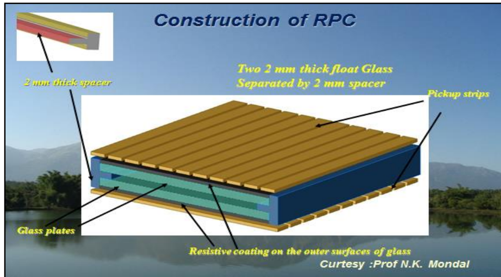
Figure 1.7: Typical RPC with pickup panels
