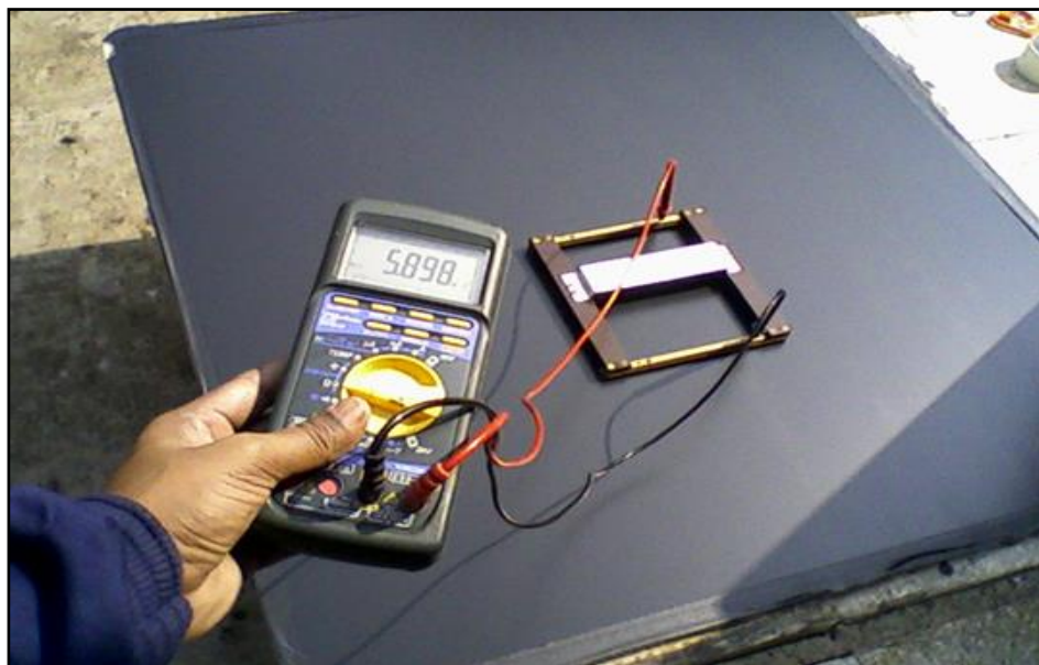
Figure 1.8: Zig to measures conductive surface resistance
