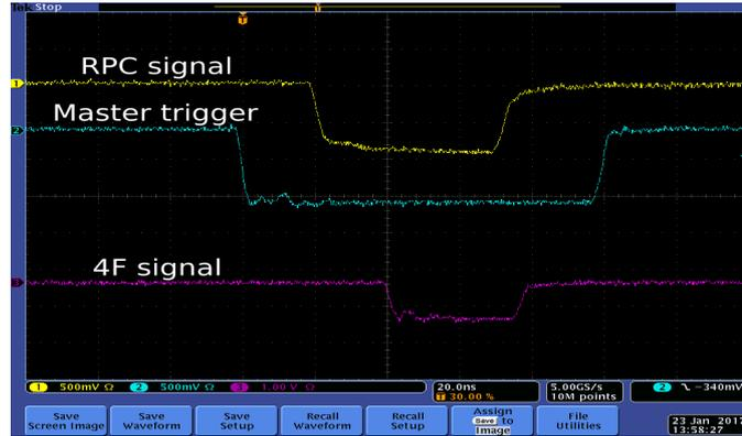
Figure 3.19: The START and STOP signals for the TDC. Displayed 4F signal was used to trigger the oscilloscope.
