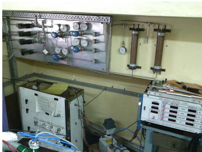
Figure 3.26: The gas mixing and the delivery unit.
