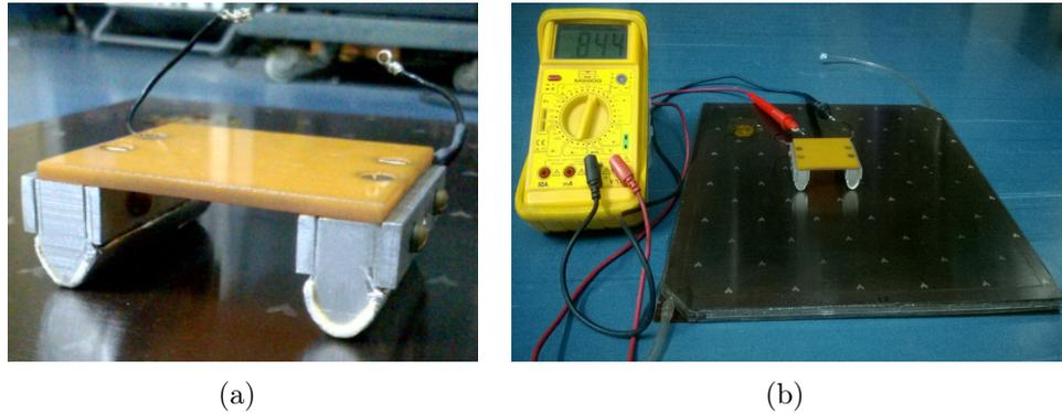
Figure 3.7: (a) The jig used to measure surface resistivity of the coated electrodes, (b) setup for the measurement.
