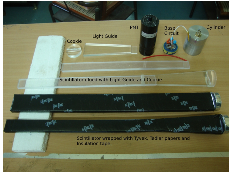
Figure 4.6: Parts of the scintillation detectors at different stages of their construction.
