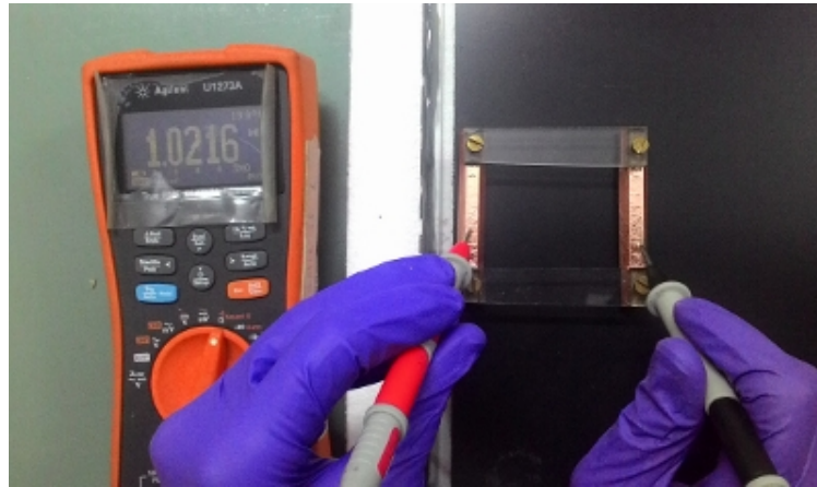
Figure 5.1: Surface resistance measurement of the electrode using a copper jig.
