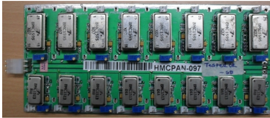
Figure 5.12: A 8-in-1 two-stage Hybrid Micro Circuit (HMC) based high speed preamplifier board.
