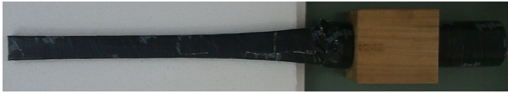
Figure 4.11: A 30 \times 3 \times 1 \text{ cm}^3 cosmic-ray paddle.
