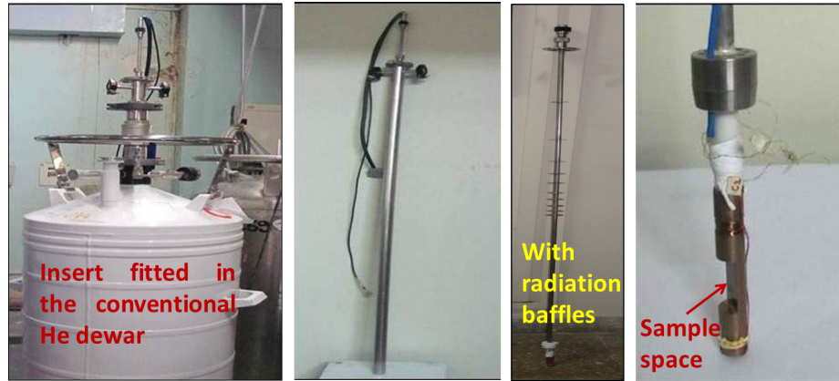
Figure 4.6: 4K Cryoinsert setup for resistivity measurements.
