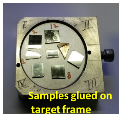
Figure 3.7: Samples placed on channeling sample holder.
