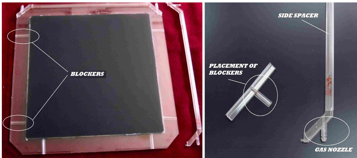
Figure 8.10: The placement of the blockers and side spacer. As shown in the left panel, two blockers are placed near each gas inlet while one blocker each are placed near each gas outlet, to ensure a proper gas flow through the sub gaps. The right panel shows a side spacer, fitted with a gas nozzle. A segment of a side spacer with a blocker attached is also shown.
