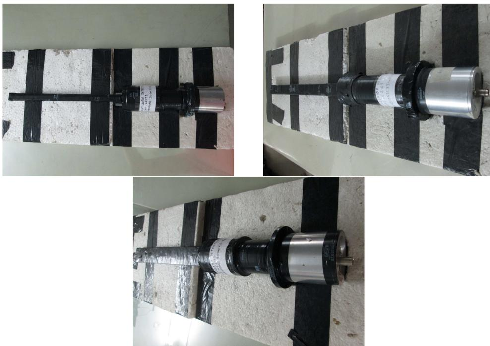
Figure 3.14: The fabricated scintillator detectors of width 1.8, 2.5 and 3.8 cm respectively.
