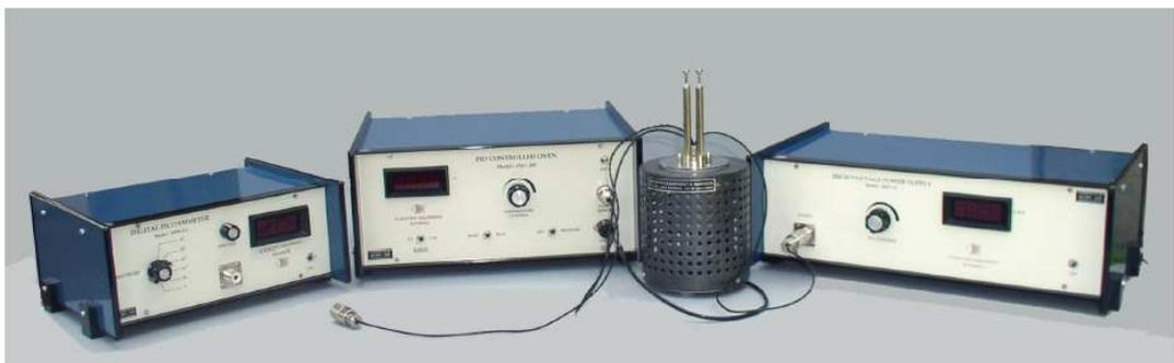
Figure 3.2: Experimental set-up for two-probe method.
