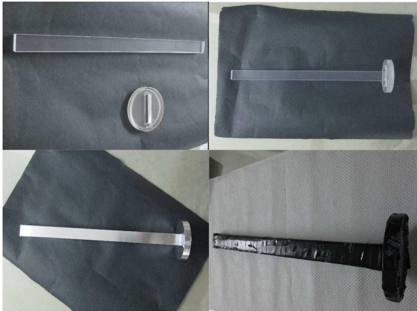
Figure 3.13: (Top-left) figure shows the paddle of 1.8 cm width and cookie before making scintillator detector. (Top-right) figure shows the paddle glued to the cookie. (Bottom-left) figure shows paddle wrapped with Aluminium for the shield from light. (Bottom-right) figure shows paddle wrapped with black paper and masked with black tape to avoid any light passing through the paddle.
