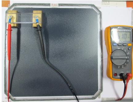
(a) RPC with jig and multimeter used to measure surface resistivity.
