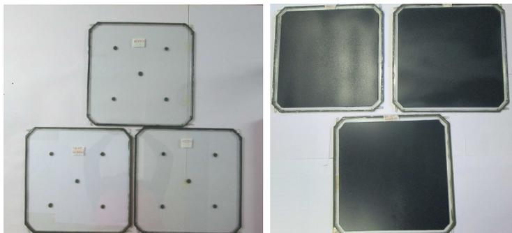
Figure 3.18: The fabricated RPCs, before graphite coating (left) and after graphite coating (right).
