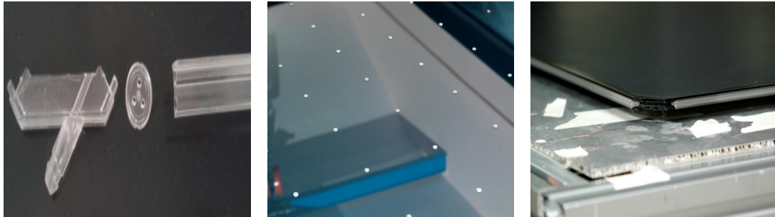
(a) Nozzle, button and side spacers (b) Electrode with button spacers (c) Side spacers fitting
