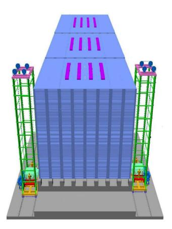
Figure 2.1: Modular structure of the ICAL detector
