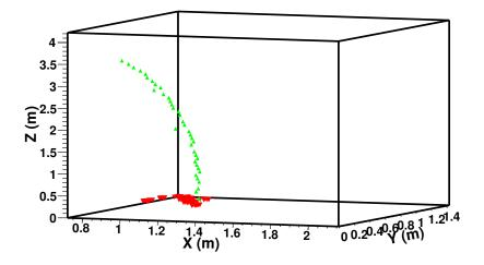
Figure 3.1: Sample track of a 10 GeV neutrino event generating a 5.1 GeV muon track and associated hadron shower in the ICAL detector
