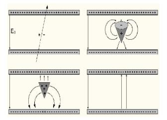
Figure 2.3: Schematic images of the development of avalanche in an RPC.Top-left panel shows ionised gas atoms by the passage of a charged particle, the avalanche size is shown in top-right panel. Bottom-left panel shows the movement of the electrons and ions to the electrode and bottom-right panel shows that the charges in the resistive layers influence the field in a small area around the position where avalanche is developed.
