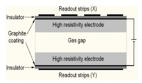
Figure 2.2: Constructional schematic of a basic Resistive Plate Chamber
