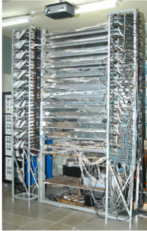
Figure 29: The prototype detector with the front-end readout electronics on either side.
