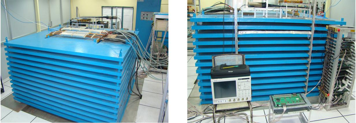
Figure 4.1: ICAL prototype detector magnet with electronics rack.
