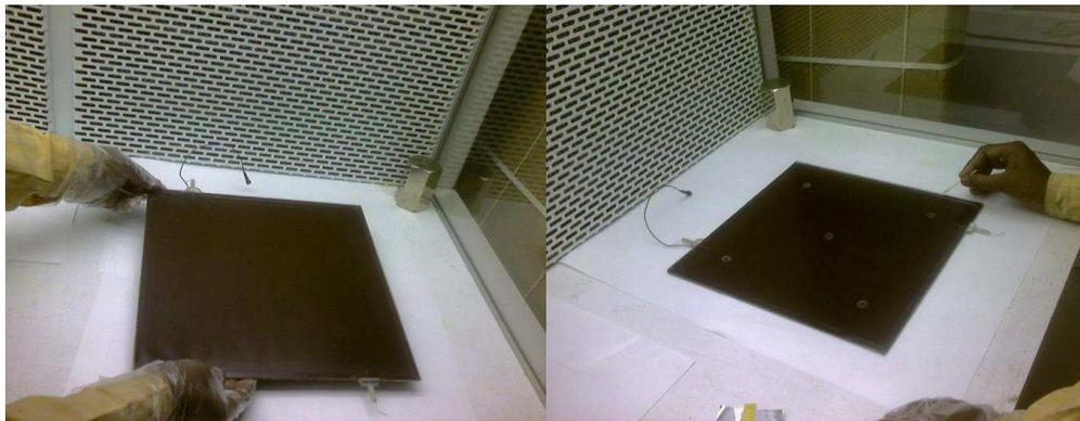
Figure 3.8: Gluing of spacers and gas nozzles on bakelite plates of  $30\text{ cm} \times 30\text{ cm}$  size.
