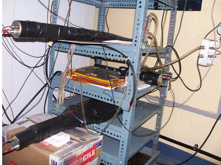
Figure 3.13: Arrangement of the scintillators and the RPC.
