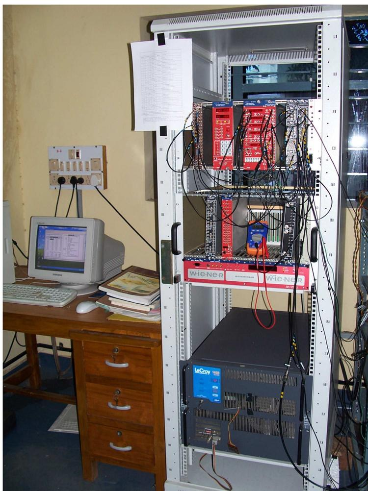
Figure 3.15: Arrangement of the power supply, front-end electronics and DAQ.
