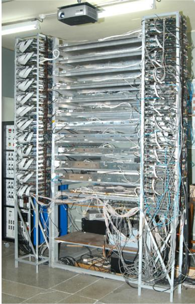
Fig. 4. Stack of INO prototype detector RPCs.
