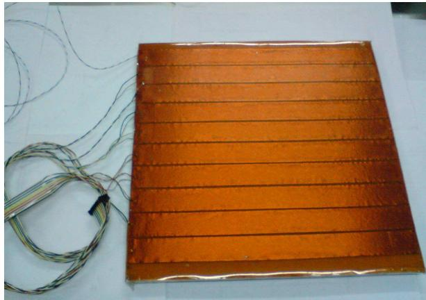
Figure 3.11: 30 cm long pick-up strip with ribbon cable.
