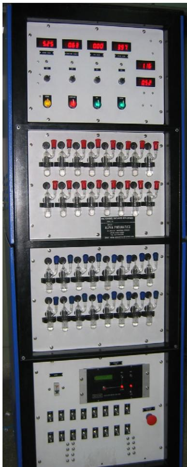
Fig. 2. On-line gas mixing and distribution system.
