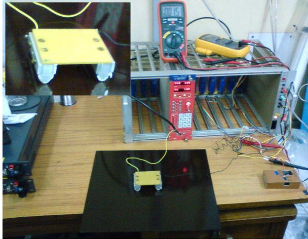
Figure 3.4: Experimental setup for surface resistivity measurement. The inset shows the figure of the aluminium jig.
