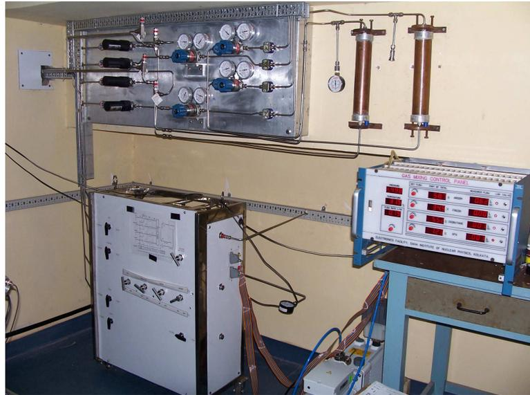
Figure 3.16: Gas mixing and delivery system.
