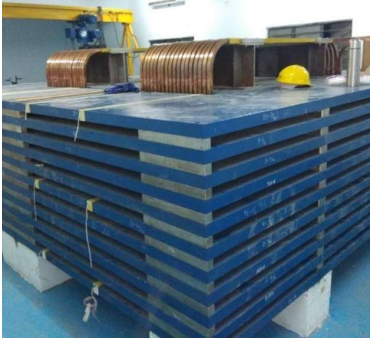
Figure 1: Magnet of the prototype ICAL detector under installation and commissioning in Madurai.
