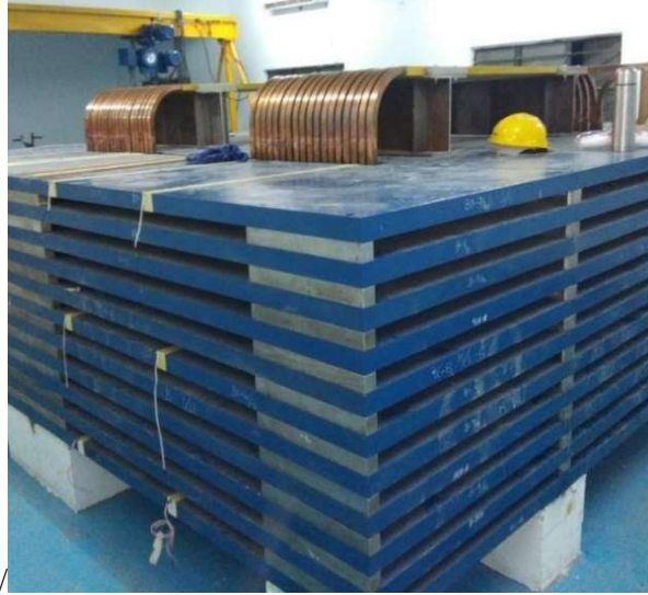
Fig.1.1 Magnet of the prototype ICAL detector under installation and commissioning in Madurai.
