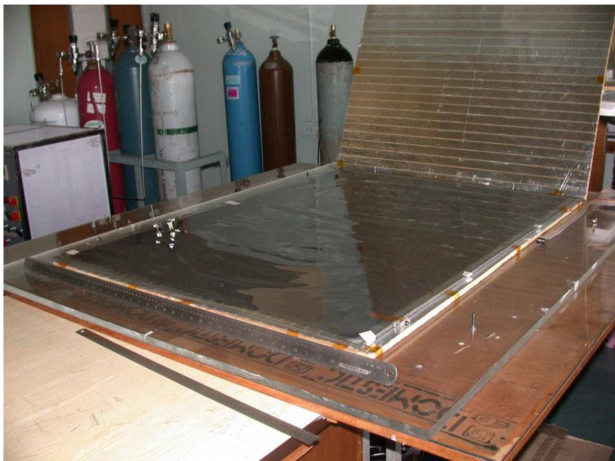
Figure 4.15: Photograph of 1 m<sup>2</sup> RPC module with its pickup strips to be used for the ICAL prototype
