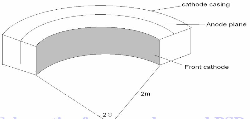
**Schematic of proposed curved PSD**
