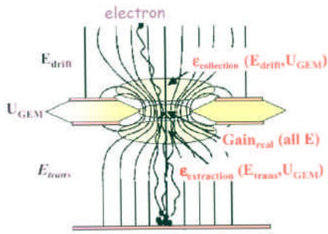
GEM foil consists essentially of a Polyimide foil (~50  $\mu\text{m}$ ), copper clad (~5  $\mu\text{m}$ ) on both side and perforated holes with typically 90-200 $\mu\text{m}$  pitch and ~60  $\mu\text{m}$  diameter.
