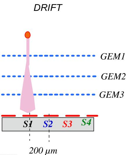
Narrow pad response function ( $D_s \sim 1$  mm):
