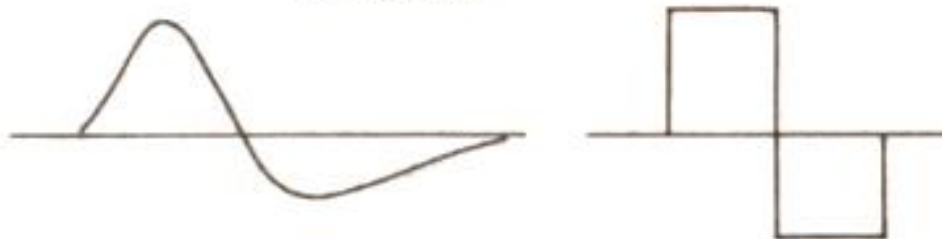
Fig. 11.2. Unipolar and bipolar pulses
