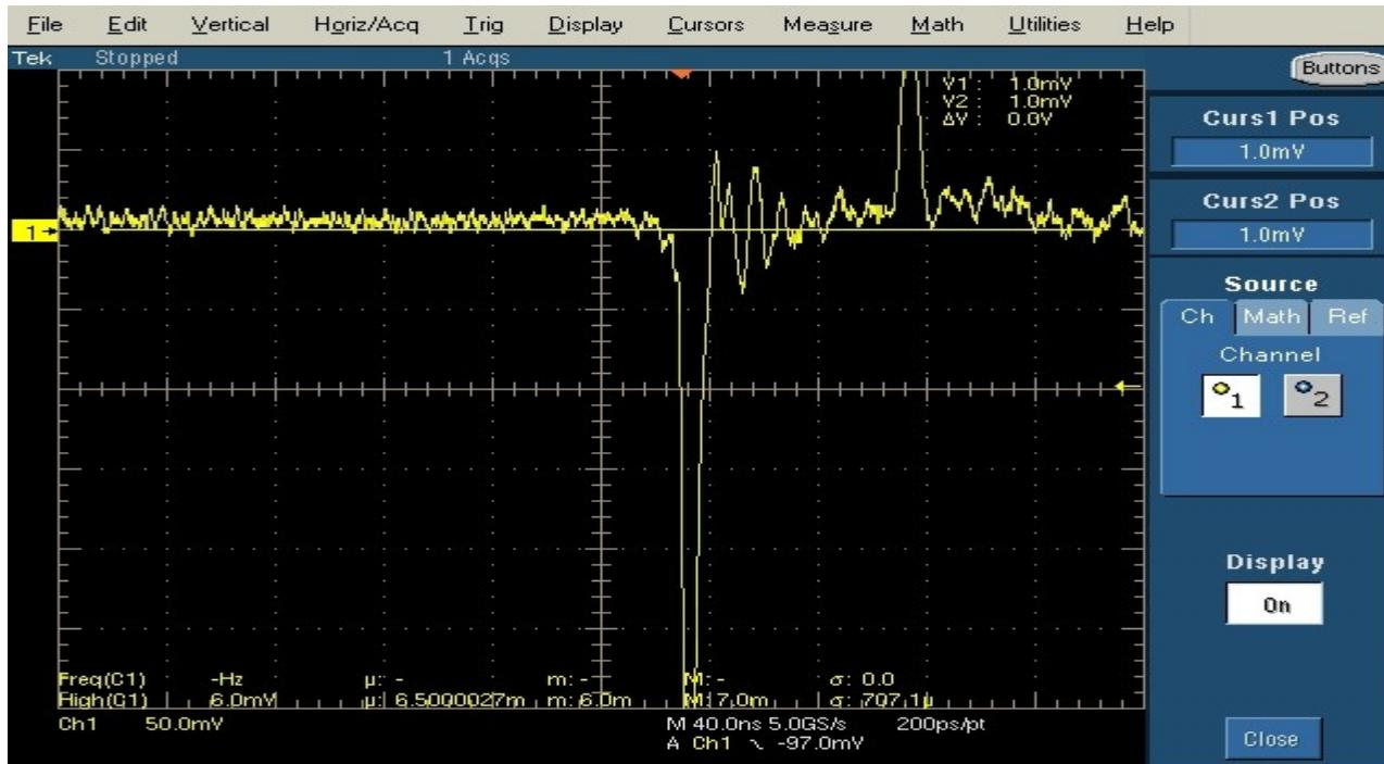
The above image is for the flattened/terminated reflected wave.
