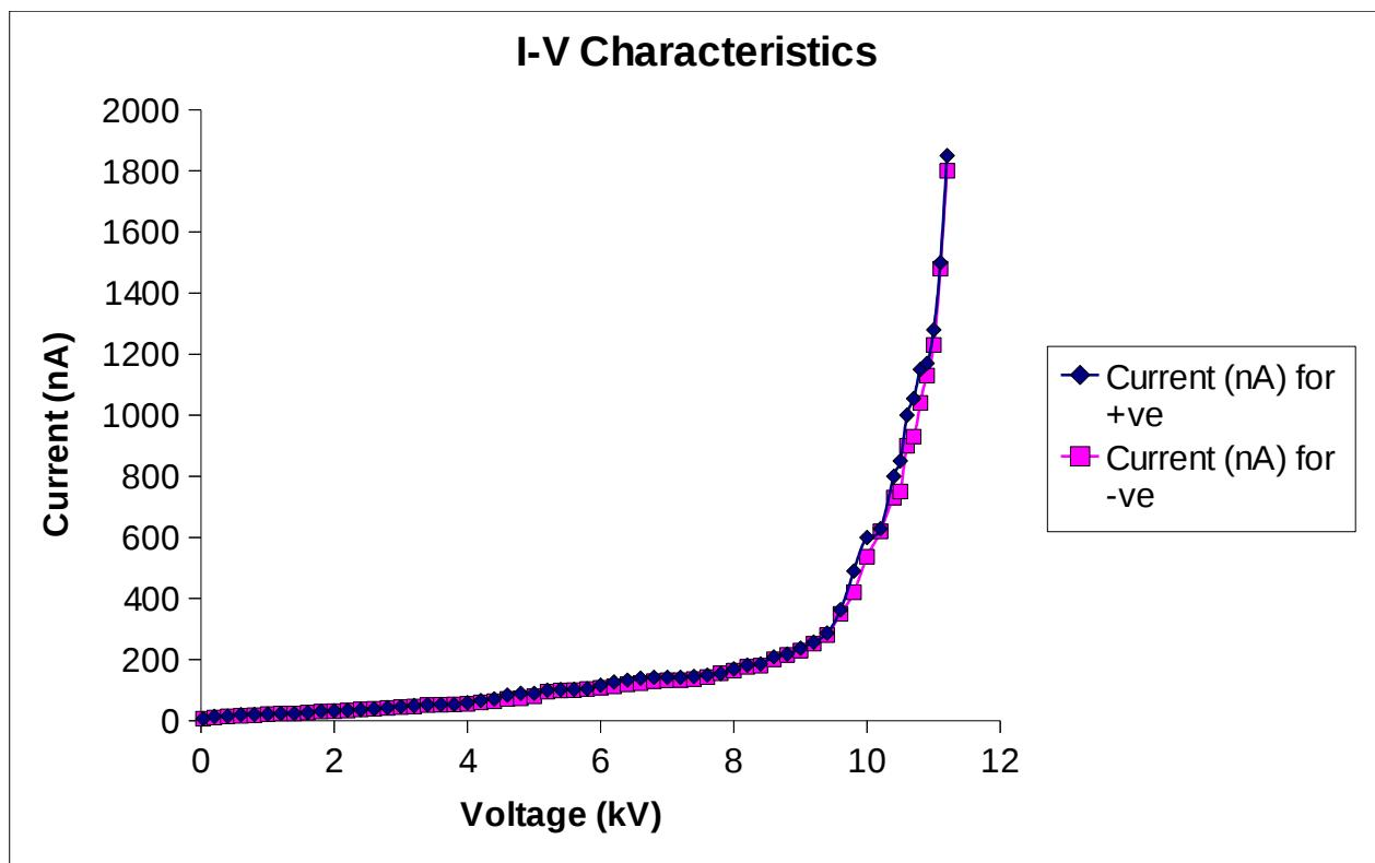
This plot shows that the breakdown voltage occurs at the high voltage ~10kV.
