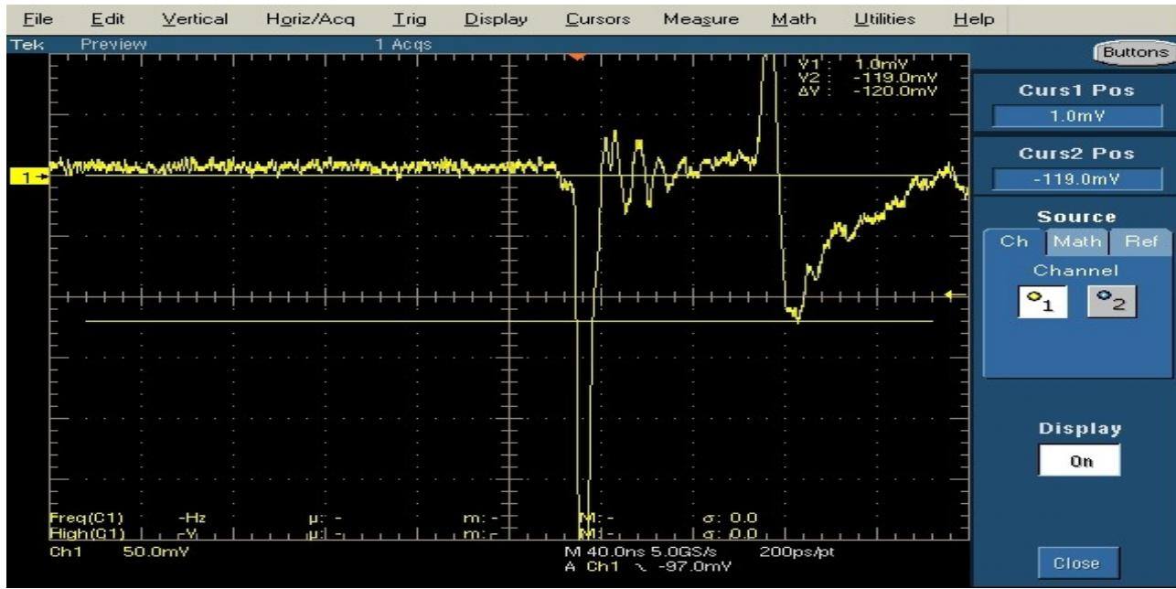
In the above image, first peak is of input signal and second peak is for the reflected wave.
