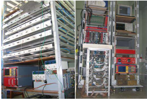
Fig. 2 A stack of large area RPCs under study (left) and the data acquisition system (right)
