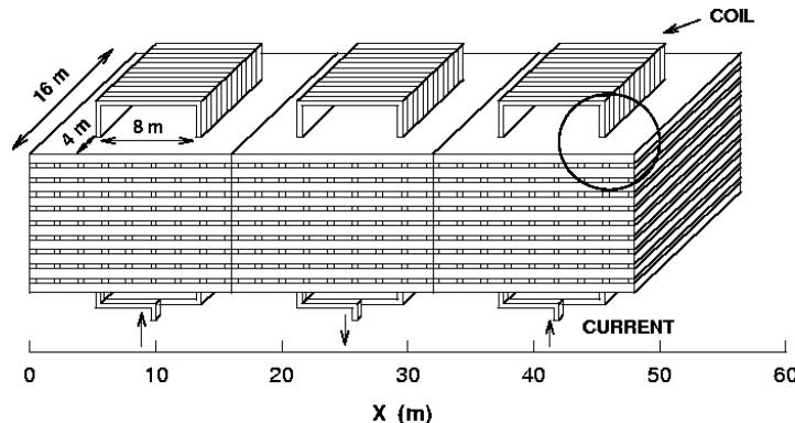
Neutrinos will interact with the iron material of the detector to produce charged particles. The iron layers will be sandwiched with the active detector material that will detect whenever a charged particle passes through it. The ICAL detector will consist of three modules of 16 kton each.
