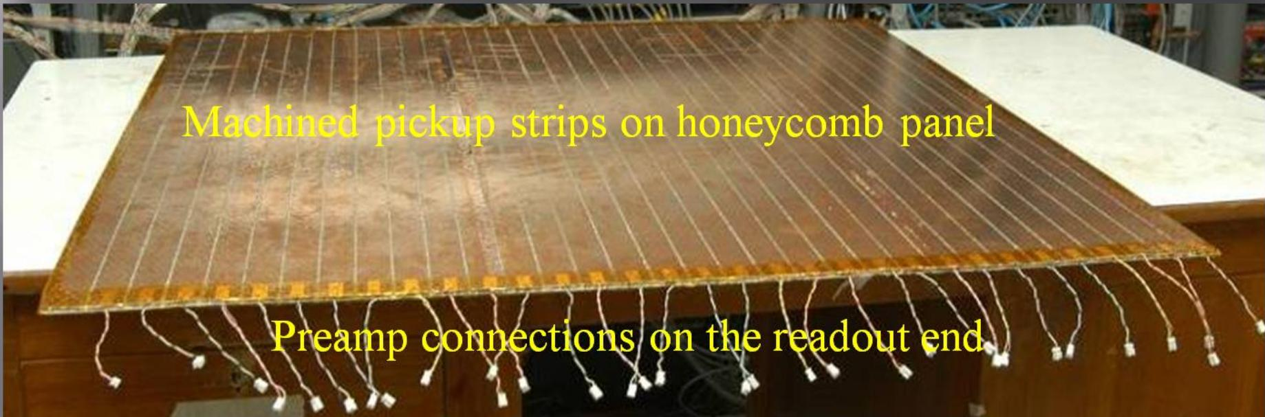
Machined pickup strips on honeycomb panel
