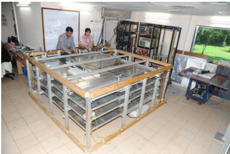
Fig 4: The 2\text{m} \times 2\text{m} prototype at TIFR (INO RPC Lab)
