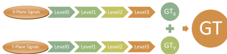
Fig.7. Complete Flow of Generation of Global Trigger Signal
