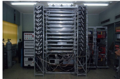
Figure 3: An RPC stack tracking cosmic ray muons
