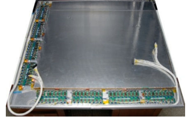
Figure 2: A prototype RPC unit shown along with its front-end preamplifiers
