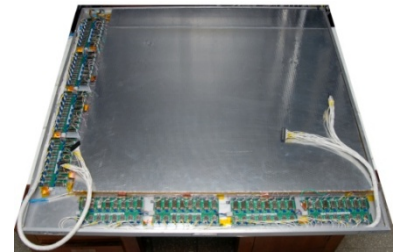
Fig. 2. A prototype RPC unit shown along with its front-end preamplifiers
