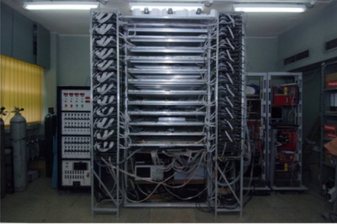
Fig. 3. An RPC stack tracking cosmic ray muons
