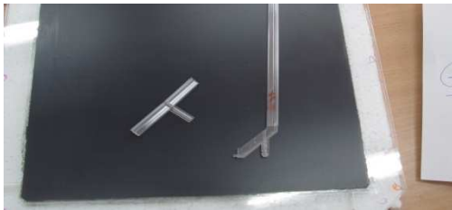
Fig 3.6: (Left) Plastic channel fitted onto an edge spacer and an edge spacer connected to a gas nozzle. Fig 3.7 (Right) The edge spacer and gas nozzle (made for the single gap RPC) fit perfectly in the gas gap of the MRPC
