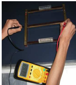
Fig3.4: Surface Resistivity of the graphite coating was measured using indigenous jig and a multimeter.
