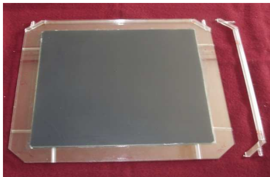
(Left) Fig 3.8: MRPC, Edge spacers and gas nozzle before the application of glue. (Right) Fig3.9: Glue being applied on all edge spacers and gas nozzles.
