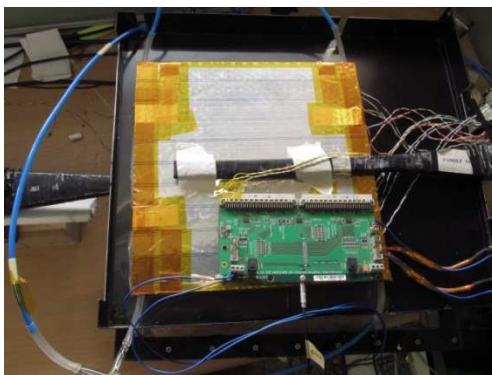
Fig 3.10: The entire setup of the MRPC including scintillator paddles, pickup panels covered with Kapton tape, gas tubes and the NINO board.
