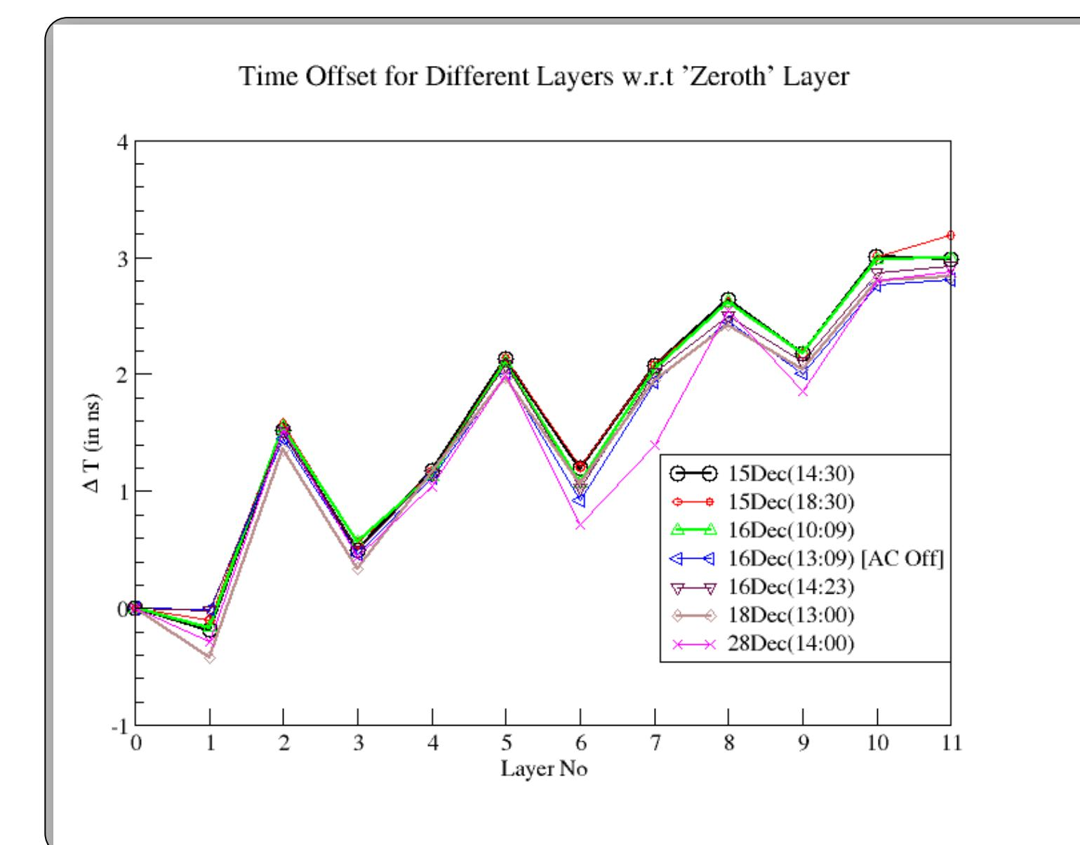
The plot shows the relative time-differences for the different layers taken over a period of time. These data were used to correct the timing data .
