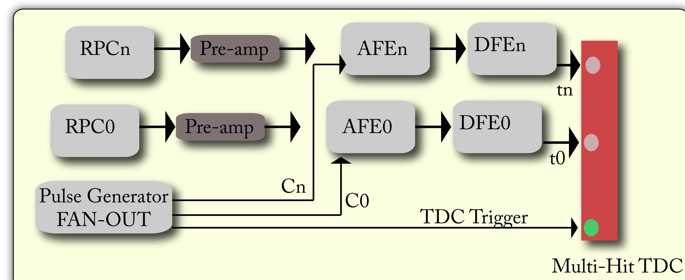
The calibration set-up is shown in the block diagram above. Since the effective contribution to the time delays come mainly from the electronics succeeding the pre-amplification stage, all calibration signals are input to the Analog Front-End (AFE) stage of the signal processing.
