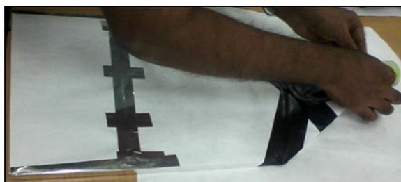
Fig.8 Scintillator wrapped in TYVEC paper
