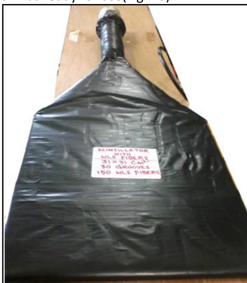
Fig.10 Scintillator(31cm x 31 cm), 150 WLS fibers, with PMT
