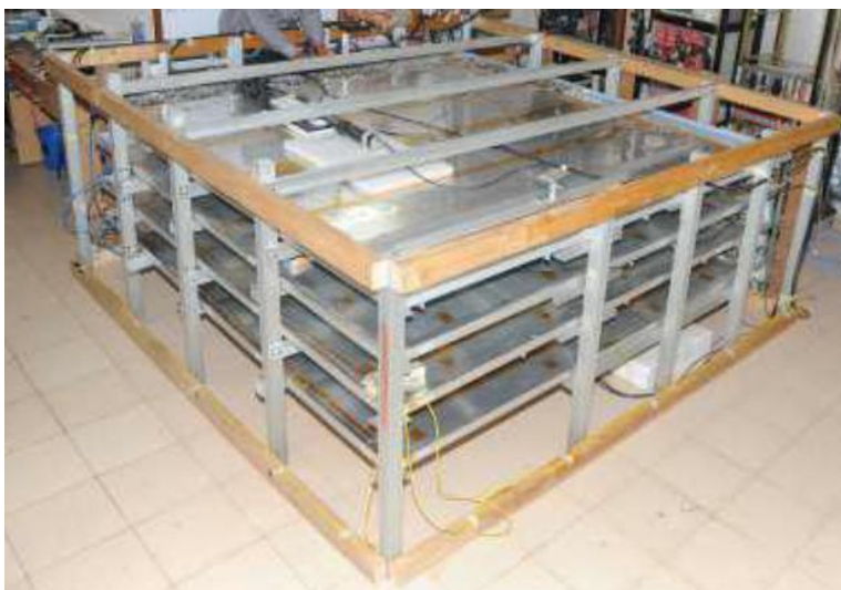
Fig.2 ICAL detector with 12 RPCs stack. Each RPC has an area of 2m x 2m with 64 pickup strips each for plane X and plane Y. This is installed in New INO Lab.
