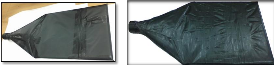
Fig. 9 Scintillator further wrapped in Tedlar sheet and then black tape
