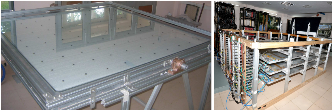
Figure 3.41: A 200\text{ cm} \times 200\text{ cm} RPC being fabricated (left panel) and three such RPCs are under test in a cosmic ray test stand (right panel).
