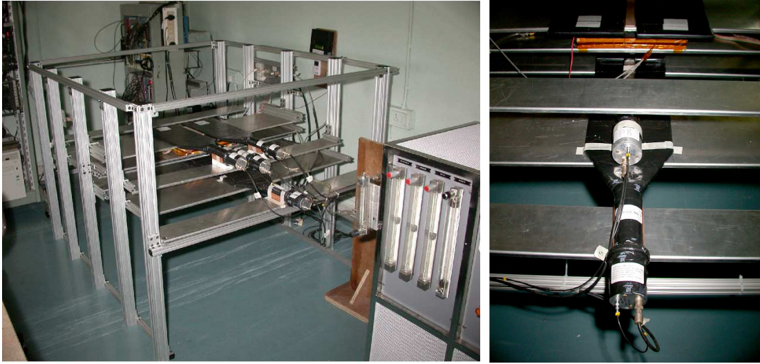
Figure 3.3: A cosmic ray muon telescope set up (left panel) and close-up view of its precise alignment along with the RPC under test (right panel). RPC is seen in bright orange colour as its pickup panels are covered with a Kapton tape. The finger (2 cm wide) paddle and a pair of veto paddles which surround it, are all mounted on top of the RPC.
