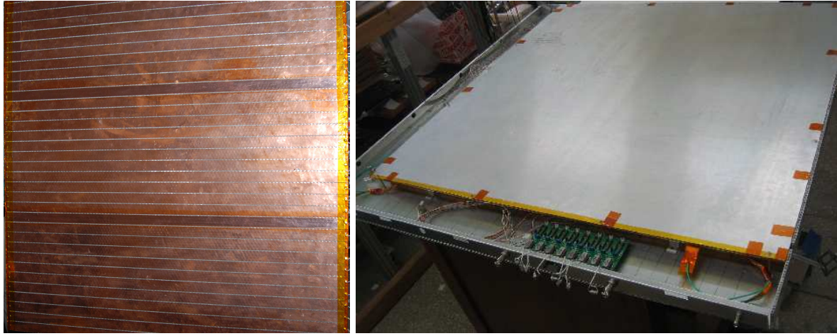
Figure 3.39: Honeycomb panel with milled copper pickup strips shown (left panel) and partially assembled RPC using aluminum honeycomb panel.
