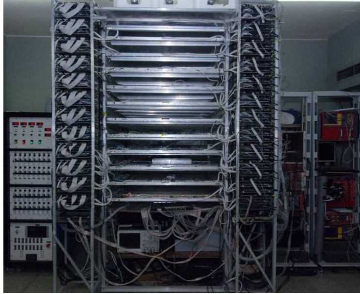
Figure 4.2: Fully installed ICAL prototype detector stack along with the gas system (left) and DAQ and power supply systems (right). The front-end electronics racks are built on either side of the detector stack - one each for X- and Y-readout planes.
