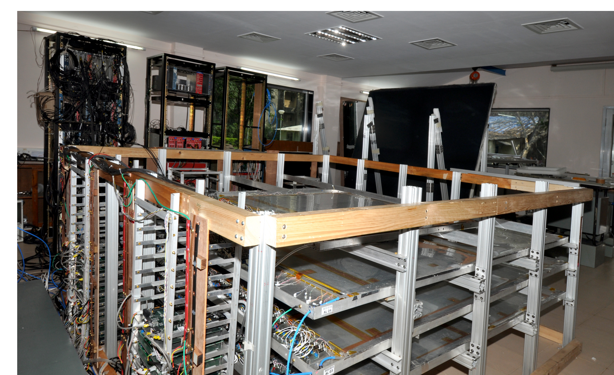
Figure: The stack of 2mx2m RPCs at TIFR, Mumbai.
