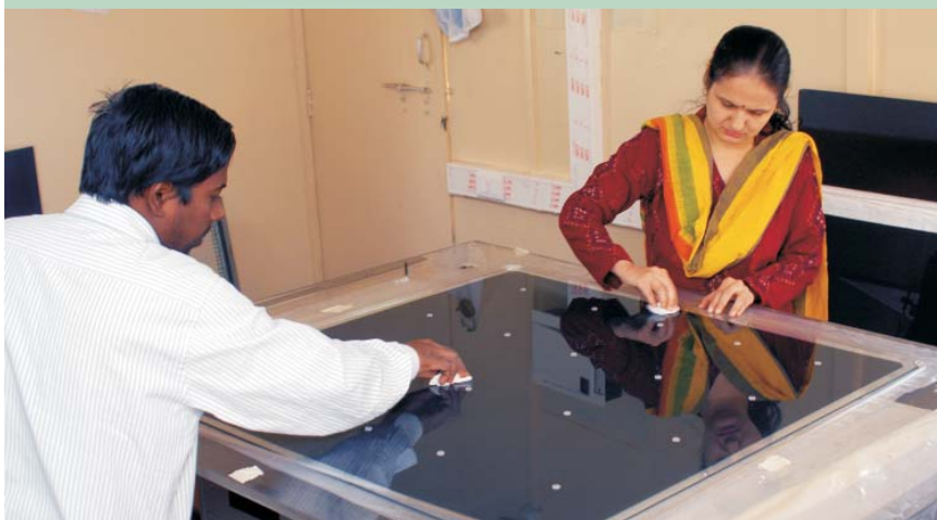
The India-based Neutrino Observatory is set to be dug into this mountain (above) in Tamil Nadu (the arrow indicates the entrance). Technicians prepare resistive plate chambers (below) for a prototype magnetized iron calorimeter detector.
