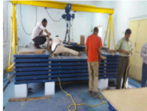
Assembly of iron plates of mini-ICAL magnet
