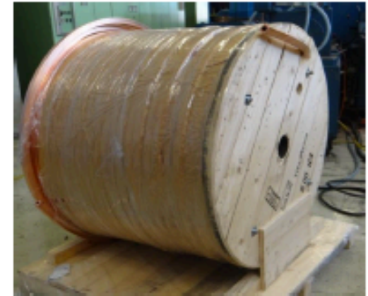
Copper Conductor Spool
