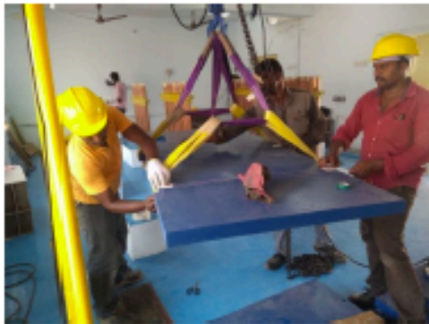
Assembly of iron plates of mini-ICAL magnet
