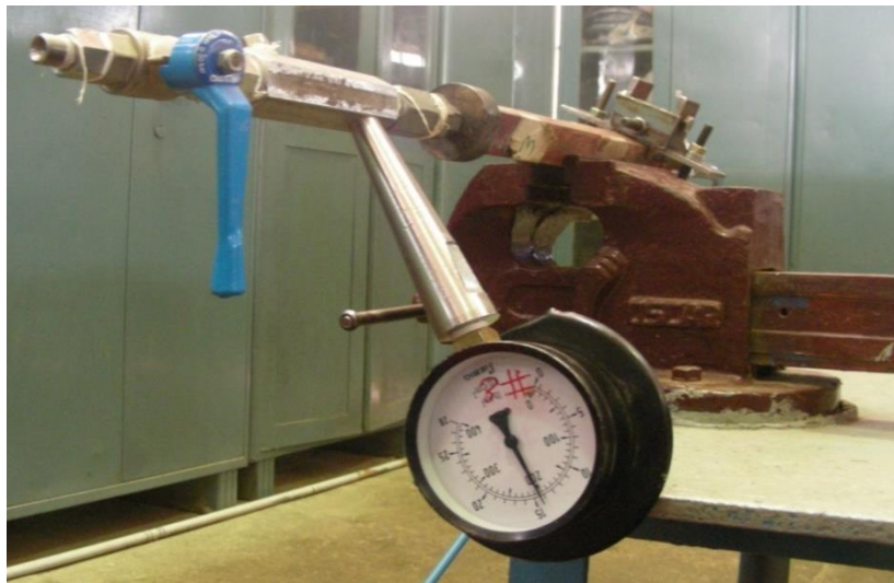
Brazing joint pressure test
