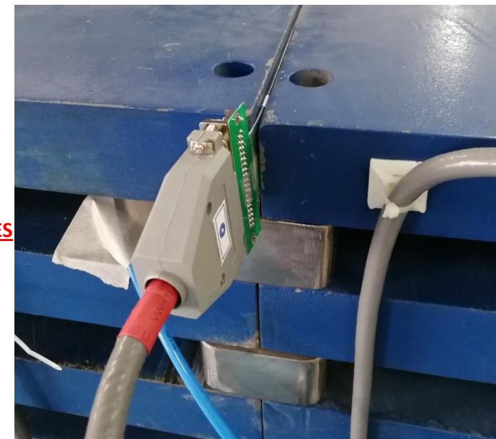
Hall probe PCB in the gap
