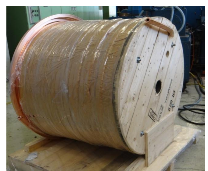
Copper Conductor Spool
