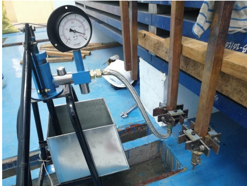
Coil hydrostatic pressure test
