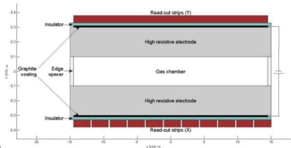
Schematic diagram of a complete RPC
