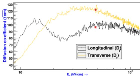
Variation of Townsend coefficient ( $\alpha$ ), attachment coefficient ( $\eta$ ), electron drift velocity ( $V_z$ ) and diffusion coefficients ( $D_l$  and  $D_t$ ) with applied field ( $E_z$ ) from MagBoltz.
