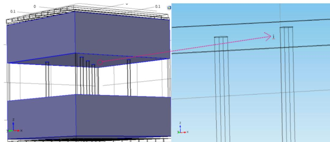
Block-shaped roughness at the inner surface of RPC plate
