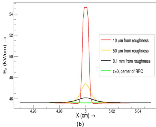
Variation of  $E_z$  with  $X$  at different distances from the block-shaped roughness from (a) COMSOL, (b) neBEM.
