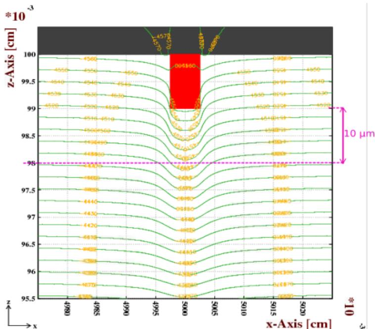
Contour plot of  $E_z$  around the block-shaped roughness.
