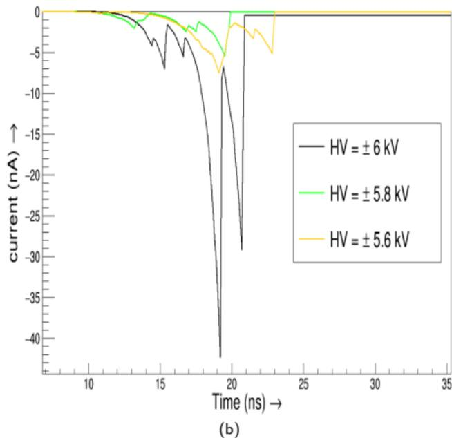
Average RPC signal for different applied voltages when 2 GeV muons are passed through (a) regular region, (b) near edge
