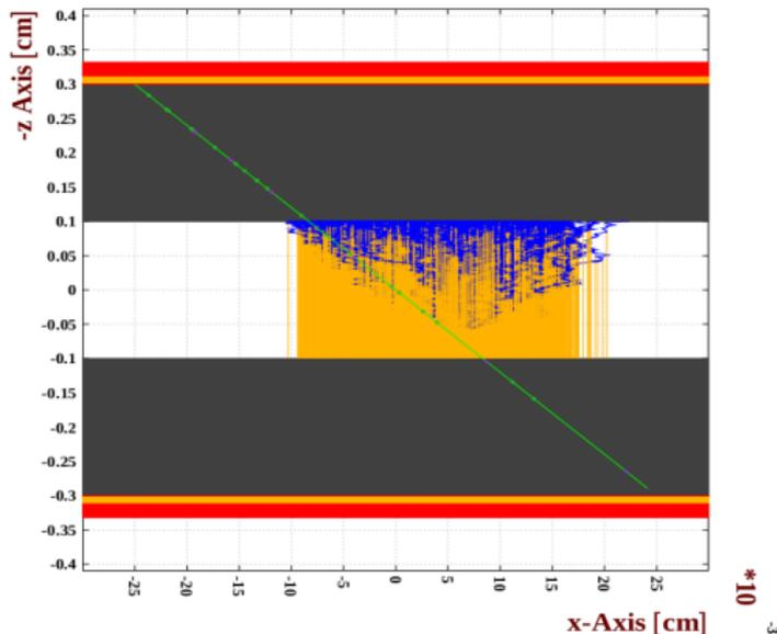
Avalanche produced due to drift of electrons and ions within RPC gas chamber
