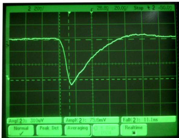
RPC signal as seen on Oscilloscope.
