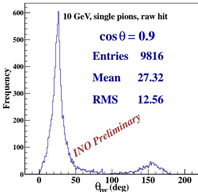
Figure 6: Distribution of reconstructed  $\theta$  ( $\theta_{rec}$  in degrees) for a 10 GeV single pion incident in the  $\cos \theta = 0.9$  direction. The small peak shows the number of events in the wrong quadrant. A cut of  $l_{min} = 2$  is required for the reconstruction.
