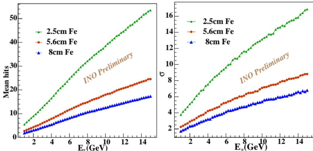
Figure 4: Mean hits (left) and  $\sigma$  (right) as functions of pion energy for some sample thicknesses.
