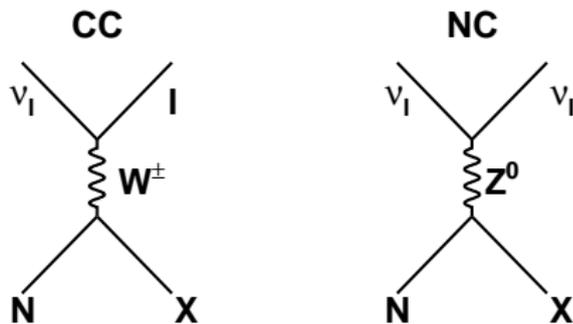
Figure 2: Charged current and neutral current interactions of neutrino with nucleons.
