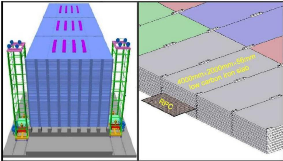
Figure 1: Schematic of INO ICAL detector with its three magnetised modules (left) and a zoom in of a section of ICAL with an RPC taken out (right).
