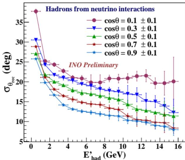
Figure 9: Resolution of reconstructed  $\theta$  ( $\sigma_{\Delta\theta_{rec}}$ ) in degrees as a function of  $E'_{had}$  in GeV for hadrons from neutrino interactions; with  $lmin = 2$  cut.
