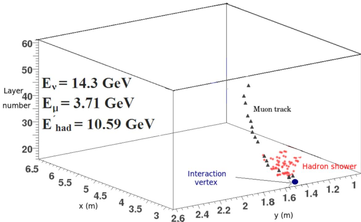
**Figure 3:** For a charged current muon neutrino interaction in INO ICAL. Net hadron energy  $E'_{had} = E_\nu - E_\mu$ , where  $E_\nu$  is the energy of the incident neutrino,  $E_\mu$  is the energy of outgoing muon.
