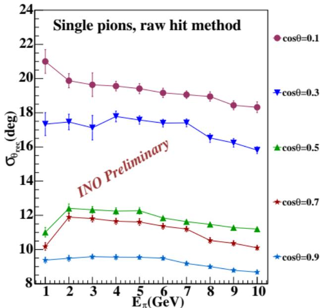
Figure 7: Resolution of reconstructed  $\theta$  ( $\sigma_{\theta_{rec}}$ ) in degrees as a function of incident pion energy for single pions; with  $l_{min} = 2$  cut.
