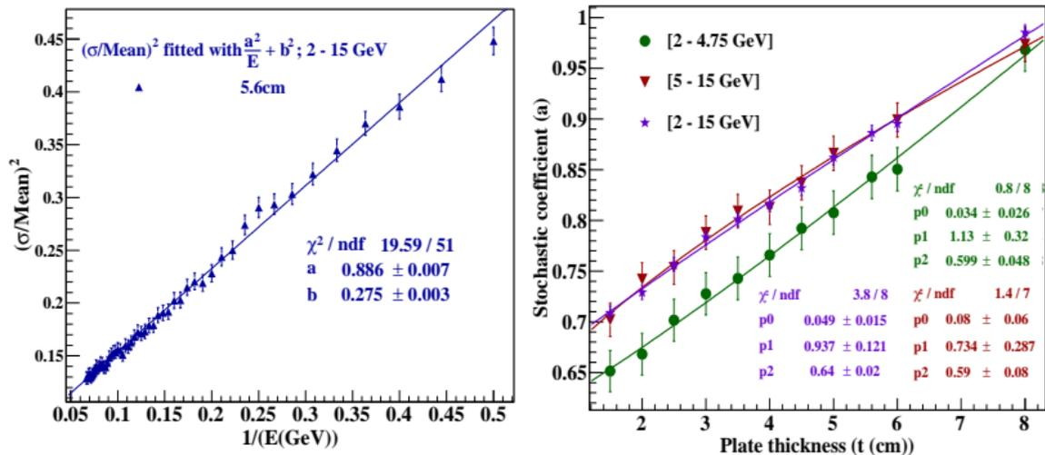
Figure 5: Hadron energy resolution in the range 2-15 GeV for the default thickness of ICAL (left). Stochastic coefficient  $a$  as a function of  $t$  (cm) in various energy ranges (right).  $p_0$  = constant,  $p_1$  = exponent which gives the thickness dependence,  $p_2$  = residual resolution
