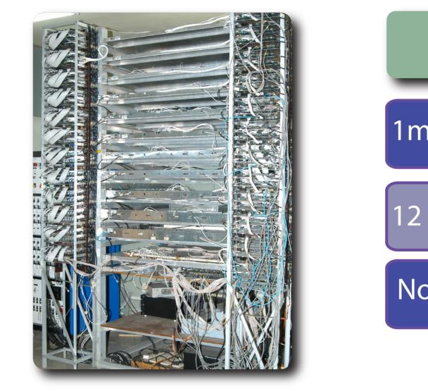
The prototype stack at TIFR is being used as a cosmic ray telescope and serves as a test bench for the detector and its related electronics<sup>2,3</sup>. Long term stability and performance studies are carried out in the stack. A VME based DAQ was developed for this set-up.
