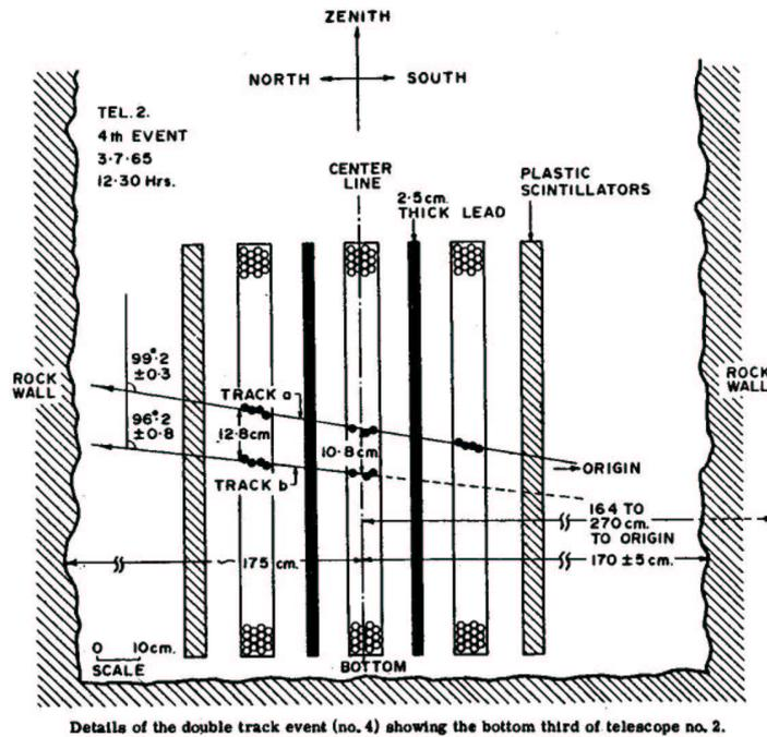
Fig. 5 An expanded view of a section of Telescope 2 in which an inelastic collision in rock of an upward-moving neutrino was recorded. The black dots are the fired NFTs.
