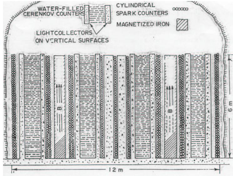
Fig. 10 The neutrino detector in Utah salt mines.
