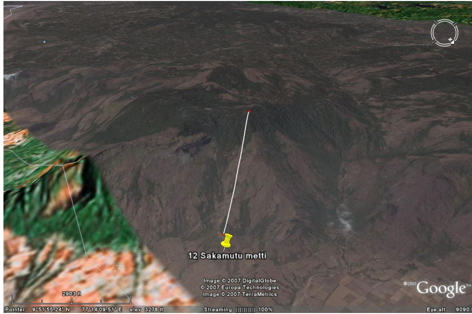
The Google Earth image shows the site Sakamutu Metti 12 with projection on the terrain of a tunnel 1344m long and overburden of 797m.
