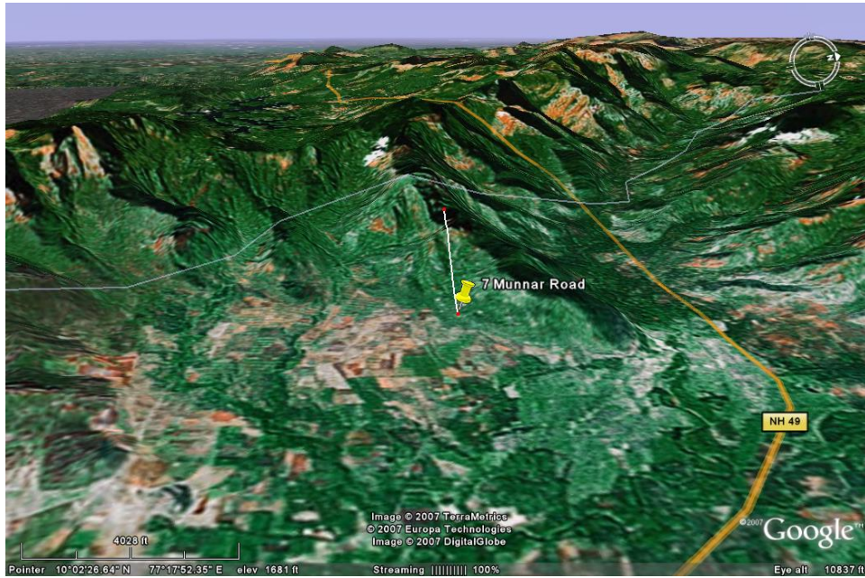
Google Earth image shows the site Munnar 7 with projection on the terrain of a tunnel 2130m long and overburden of 536m.
