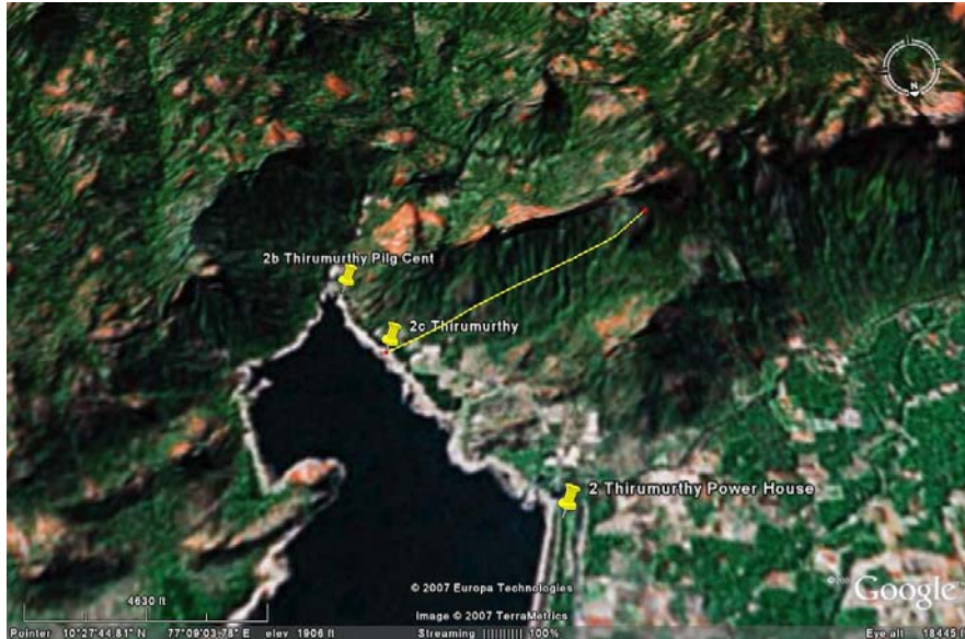
The Google Earth image shows the site Thirumurthy 2c with projection on the terrain of a tunnel 2000m long and overburden of 630m.
